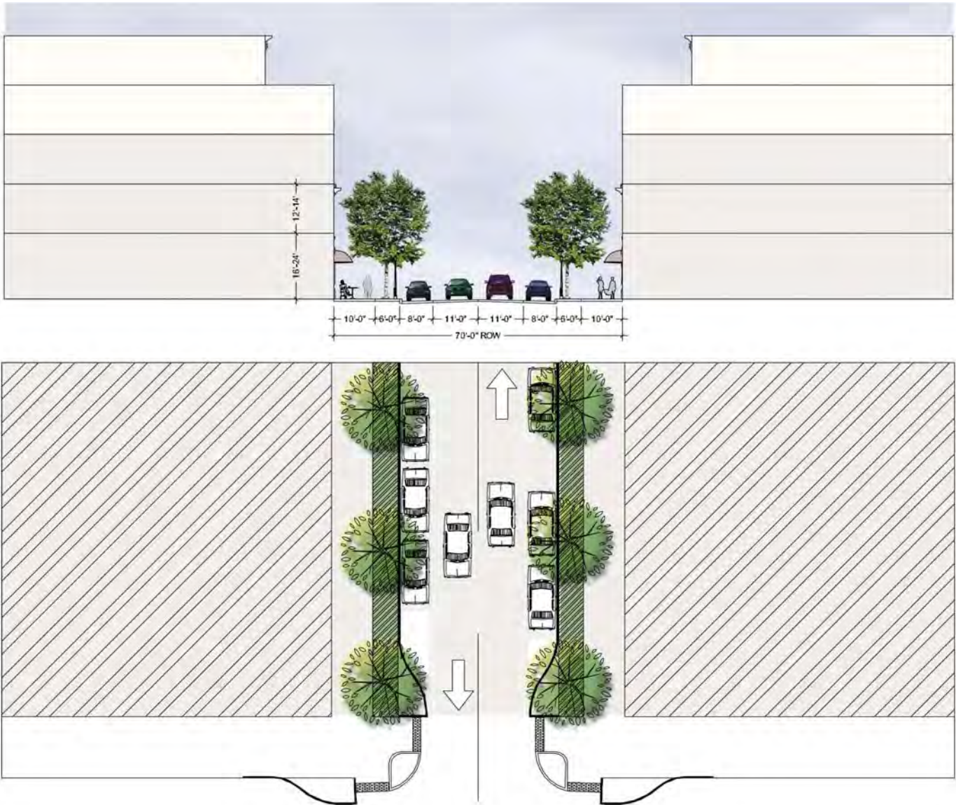
Figure 14: Section, Backstreets Option 1: Back streets would run parallel to or perpendicular to Manchester Road and would serve as relief routes for Manchester Road as well as streets serving retail, office, or residential uses throughout the study area. The recommended street sections call for one travel lane in each direction, a landscape zone of six feet between the travel lanes and areas of development, and sidewalk areas of at least 10 feet in width to facilitate retail and commercial activities. The streets should include bulb outs at intersections to shorten the distance pedestrians must travel from one side of the street to another. Parking may line the street on both sides in a parallel fashion or may orient in an angled fashion on one side, in order to increase the total number of parking spaces. Buildings of up to four stories may flank back streets. The exact form and orientation of buildings along back streets would depend on market forces and individual redevelopment concepts.
