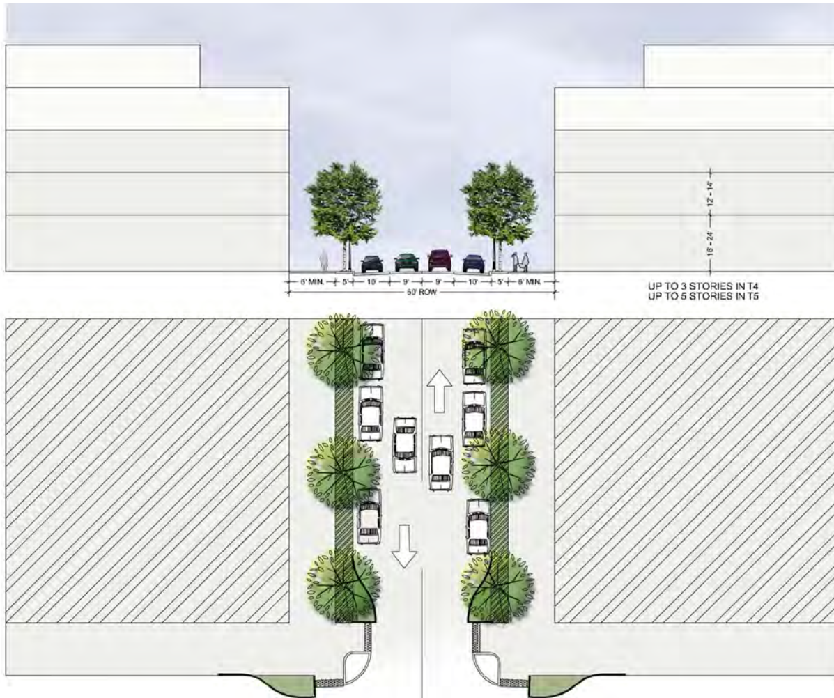
Figure 21: Section, Residential Street: Residential streets would serve as lower volume streets accessing residential developments in close proximity to Manchester Road. These streets would feature a lane of travel in each direction and parallel parking on each side. A landscape strip would separate the parallel parking area from sidewalks on either side.
