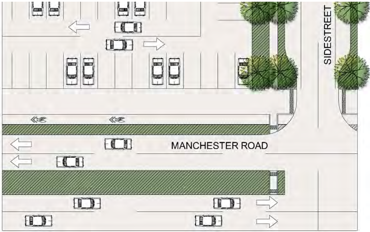
Figure 25: Section, Side Street at Left Turn Locations: This section in plan and elevation view depicts the recommended design for the intersections of the main boulevards along Manchester Road and the side streets running north-south.
