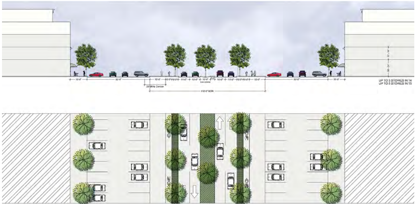
Figure 19: Section, New Boulevard: The “New Boulevard” street section reflects the recommended design for most of Manchester Road, between Baxter and Old State. As mentioned elsewhere in the master plan, the boulevard would over time include a landscaped median as redevelopment proceeds along the corridor in order to improve aesthetic quality and improve safety. A combined sidewalk and bike lane would be separated from the main travel lanes on either side of Manchester Road by a landscape buffer. A shallow bay of parking would potentially flank buildings on either side of the road, but the majority of parking would locate to the rear or side of individual buildings.
