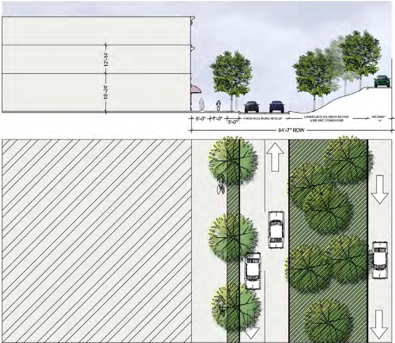
Figure 17: Section, Frontage Road (Woods Mill Road): Woods Mill Road represents a frontage road along the west side of Route 141 in Manchester. The section below outlines the recommended setbacks from Route 141 and the setbacks from buildings to Woods Mill Road.
