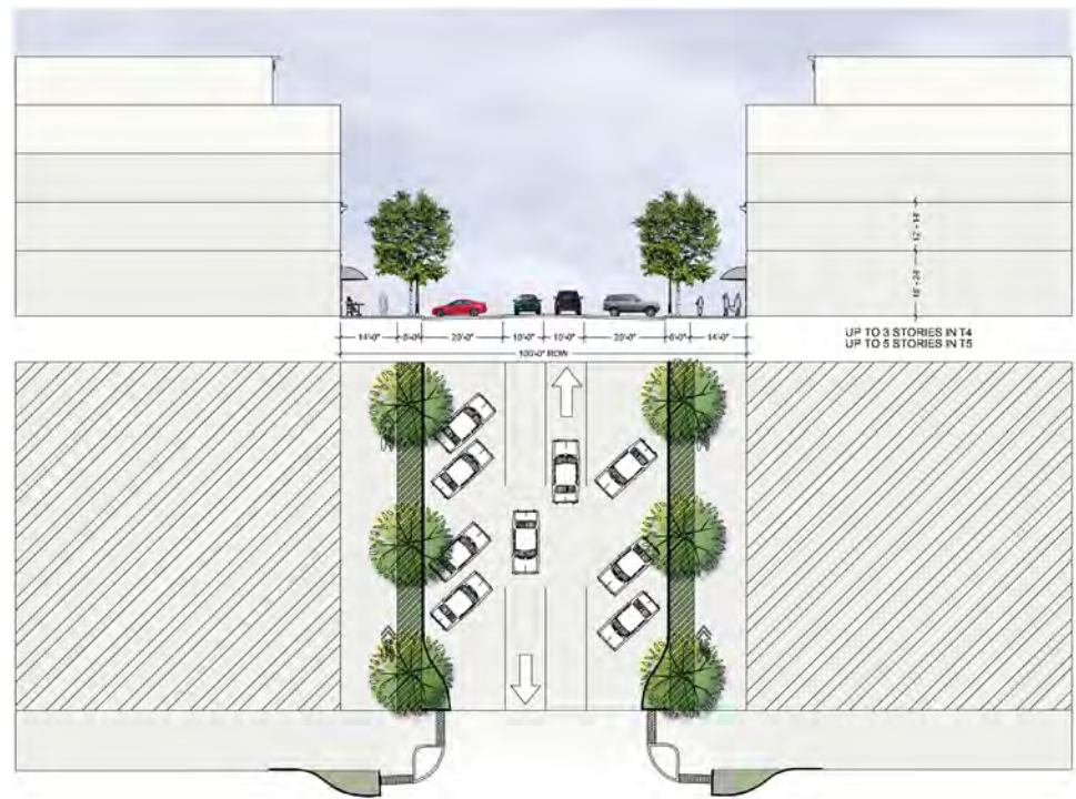
Figure 18: Section, Main Street: The “Main Street” section represents the recommended design for primary main streets in the various town center districts along the Manchester Road corridor. The street section recommends angled parking along either side of a two lane road in order to increase the number of parking spaces along the street. A minimum 10-foot wide sidewalk along the main streets would help facilitate outdoor dining and accommodate greater numbers of pedestrians compared to side streets or back streets. Landscaping including street trees will line the Main Streets. The plan anticipates buildings of up to five stories in height on either side of Main Streets.
