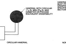
HANDRAIL THAT IS NOT CIRCULAR MUST PROVIDE "EQUIVALENT GRASPING SURFACE" TO THE SPECIFIED CIRCULAR CROSS SECTIONS
